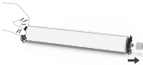
3 Remove all the debris on the main brush.
